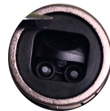
Figure 4-3: QUAD connector door partially opened
