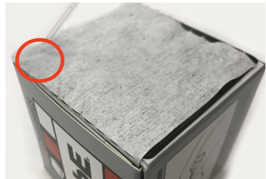
Figure 4-12: Applying cleaner to the QbE Box
