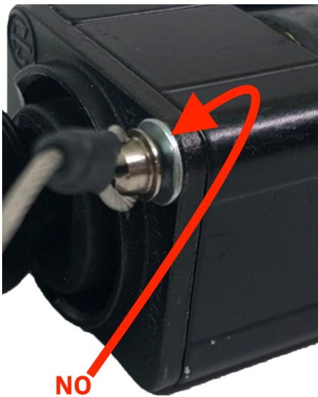
Figure 4-5: Coupler with Washer present
